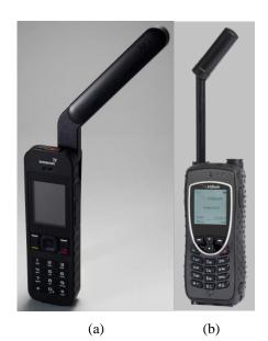
Figure 2. Satellite Mobile Phones: (a) Inmarsat IsatPhone 2 and (b) Iridium Extreme 9575
