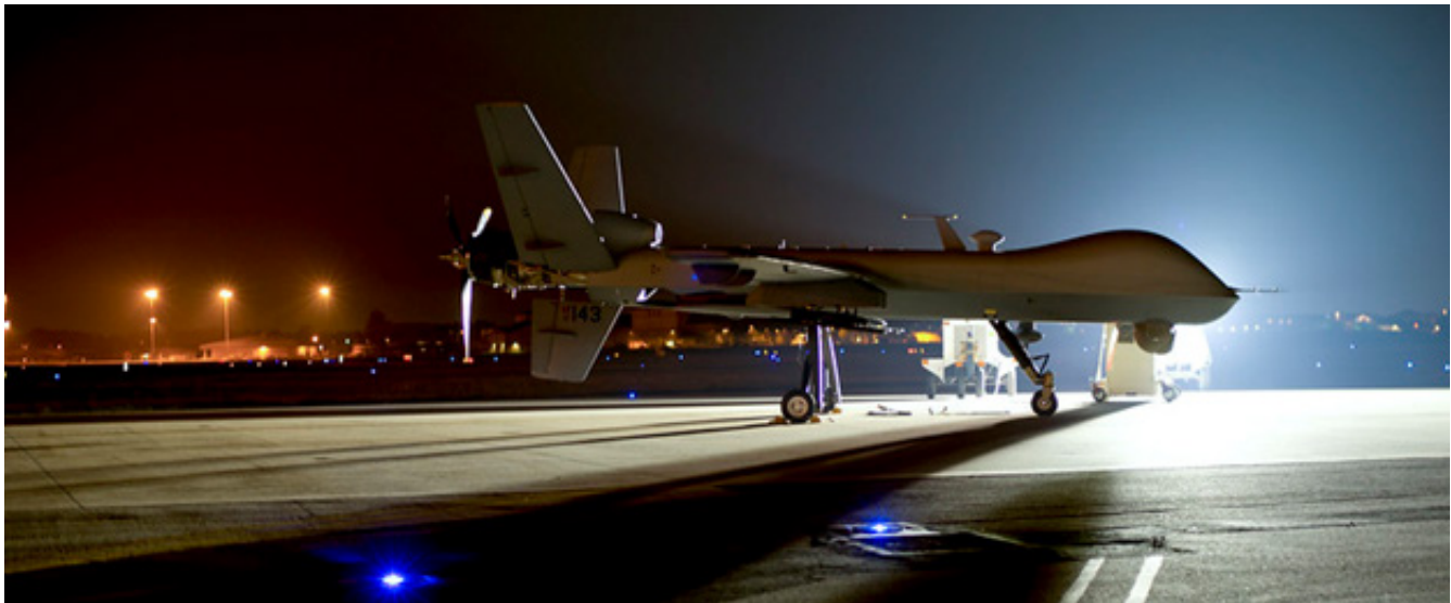
AN MQ-9 REAPER SITS ON THE FLIGHT LINE AT HURLBURT FIELD FLA., APRIL 24, 2014. THE MQ-9 REAPER IS AN ARMED, MULTI-MISSION, MEDIUM-ALTITUDE, LONG-ENDURANCE REMOTELY PILOTED AIRCRAFT THAT IS EMPLOYED PRIMARILY AS AN INTELLIGENCE-COLLECTION ASSET AND SECONDARILY AGAINST DYNAMIC EXECUTION TARGETS. (U.S. AIR FORCE PHOTO/STAFF SGT. JOHN BAINTER)
